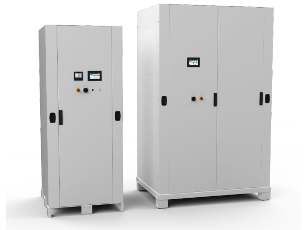
Figure 10: REGATRON's liquid-cooled system solutions up to IP54 with various power levels, e.g. 54...162 kW (left) and 216...324 kW (right). The remote control unit RCU, indicator lights, emergency stop button, and main switch allow the user to operate the system on the enclosure's front door.
