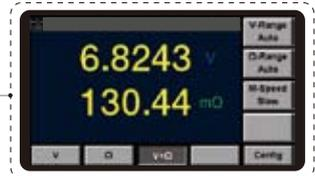
High speed simultaneous resistance and voltage measurement.
