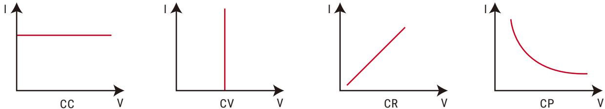
IT-M3300 also provides CC+CR/CV+CR/CV+CC/CC+CV+CP+CR four combined operation mode, which can be applied to the test requirements of various occasions.
