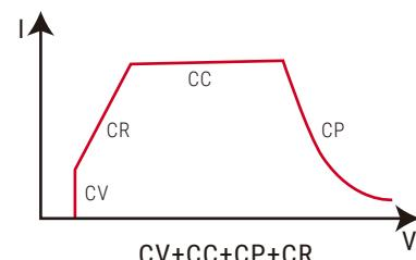
CV+CC+CP+CR mode can be applied to test lithium-ion battery charger, to gain complete V-I charging curve. In addition, when protection circuit of DUT is damaged, it can auto switch to avoid damage.
