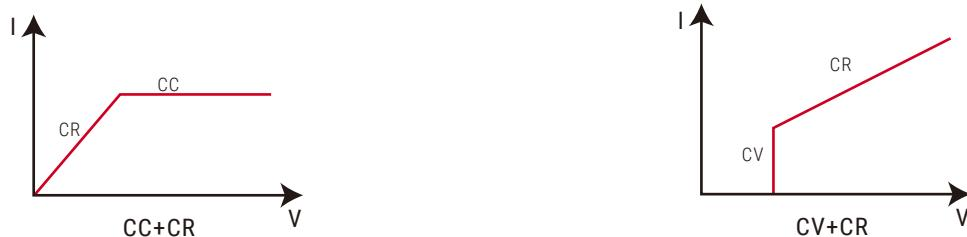
CC+CR mode can be applied to OBC feature test of voltage limit, feature test of current limit, constant voltage accuracy test, constant current accuracy test, to prevent over current protection.
