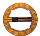
Pic A. Heating of packaging device to seal plastic bags filled with air
