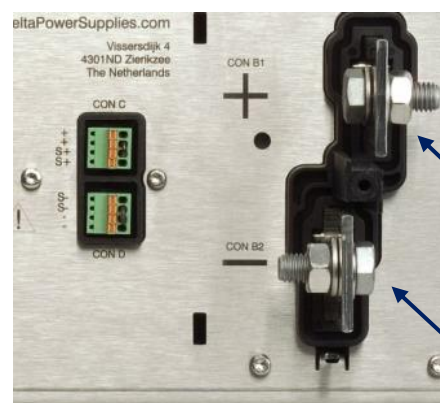
Figure 7.3: The two DC power terminals CON B1 and B2. CON C and D are the sensing connectors.
