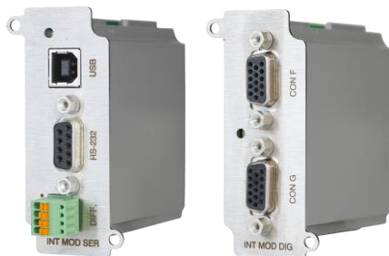
Figure 9.6: Left: Serial programming, Right: Digital I/O
