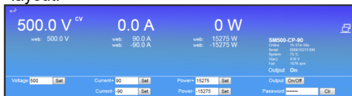
Figure 9.1: Front console for setting of the output and monitoring various parameters.
