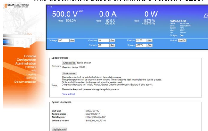
Figure 6.11: Via the web interface the downloaded firmware package can be uploaded to the unit
