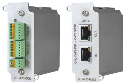
Figure 9.7: Left: Isolated contacts, Right: Master/Slave
