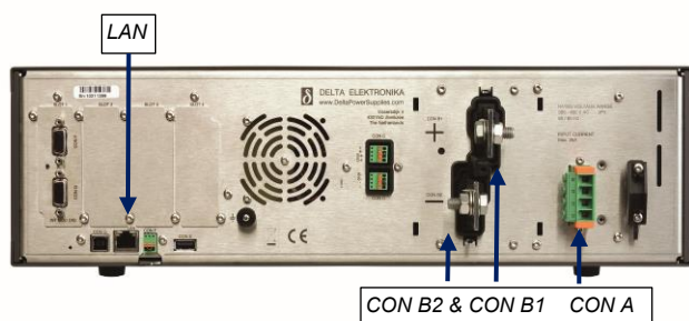
Figure 5.2: Connections on the rear side
