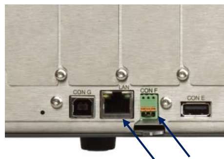
Figure 7.6: The location of the LAN-connector (left) and the Interlock connector (right) at the rear panel
