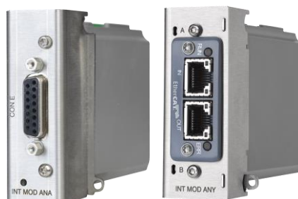
Figure 9.8: Left: Isolated analog programming, Right: Anybus carrier
