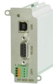
fig 8 - 7 Serial & USB Programming Module.
