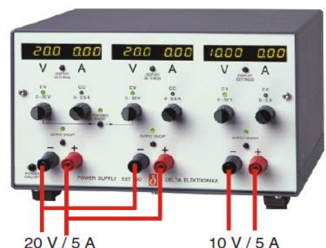
fig. 3 - 4 Parallel Tracking Mode
