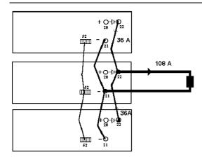
Figure 1. Current share connection with series diode.
