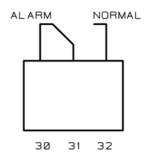
Figure 3. Alarm contact.
