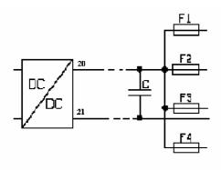
Figure 2. Connecting multiple loads.
