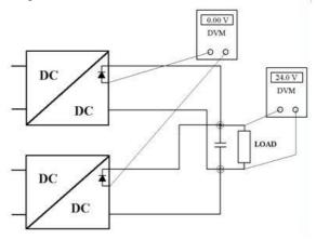
Figure 5. Adjusting output voltage measure at +Test or pin 8 on the H15 connector.
