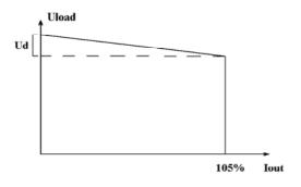
Figure 4. Load regulation with voltage drop
