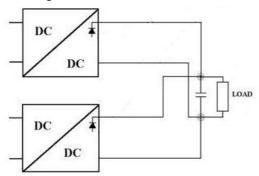
Figure 3. Parallel connection, with optional capacitor.
