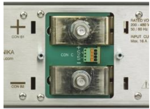
fig 6 - 3 The two DC power terminals CON B1 and B2. In between them the sensing connector.
