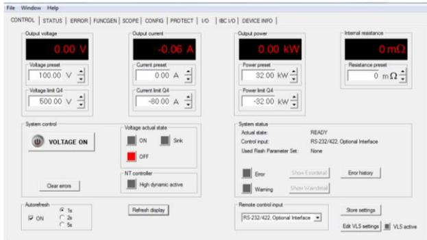
Remote connection via PC interfaces: E.g. RS232 and further interface options.
